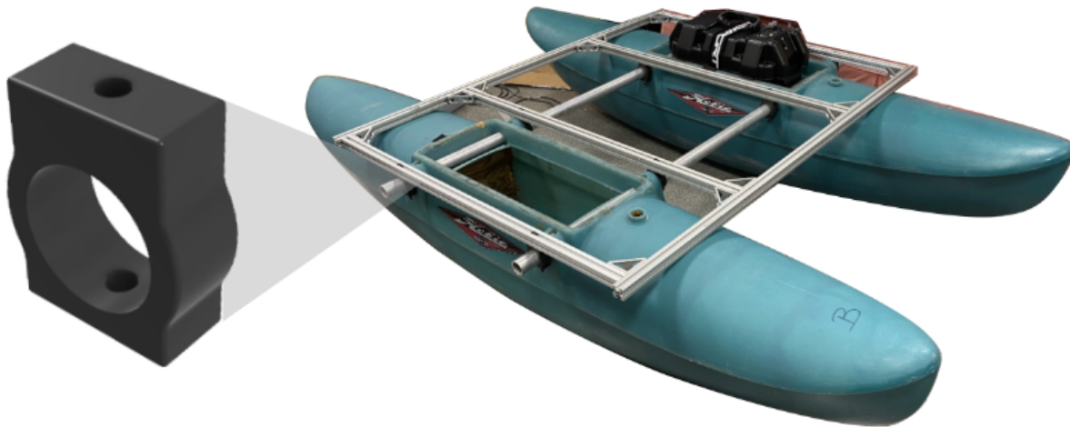
Fig. 5. 8020 frame and aluminum tubing connects the two hulls and provides a mounting platform for the marine plywood. The 8020 and aluminum are connected via a custom 3D printed spacer.
