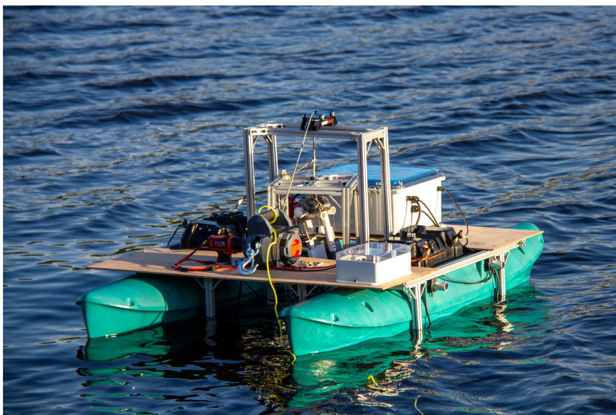
Fig. 19. The fully integrated system during outdoor river testing at Magazine Beach
